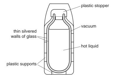
Which methods of thermal energy transfer are the silvered walls designed to reduce?
